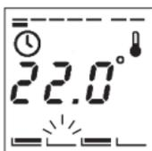
Under timer programmeringen P2, P3, og P4, indikerte blinkingen
